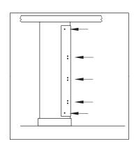
5. Drill 1/4" diameter holes through 1/2" thick panel using hole pattern of Alcove Joggle Brackets (mounted to U-channel on stile) as template.
