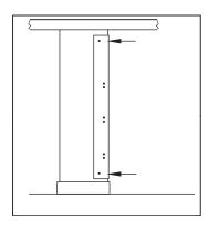
6. Use 1002499 Torx Screws - 7/16" to secure Alcove Joggle Bracket to 1/2" Thick Panel.
